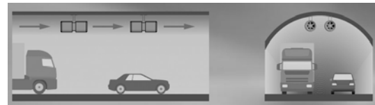
Fig. 1. Schematic diagram of Dunnae tunnel with jet-fans.
